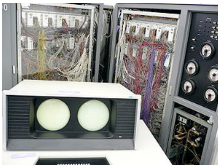
Figure 9. CDC 7600 computer (internal wiring and dual-screen console). (Source: http://en.wikipedia.org/wiki/File:Personable_Computer.jpg )
