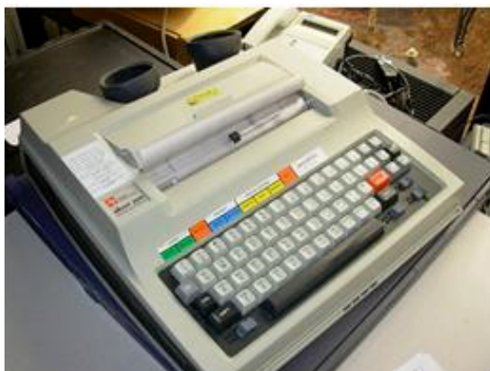
Figure 14. Texas Instruments Silent 700 terminal with acoustic coupler and thermal printer. (Source: http://www.flickr.com/photos/hckhckhck/124699193 )
