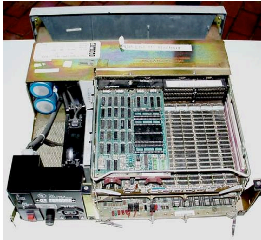
Figure 15. Inside view of an LSI-11/23. (Source: http://en.wikipedia.org/wiki/File:DEC_LSI11-23.jpg )
